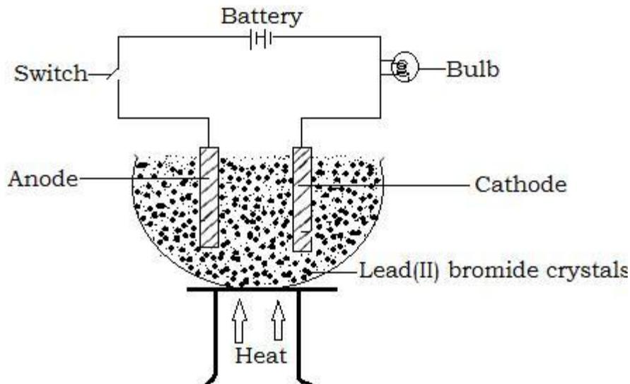
When carbon electrodes are dipped into **solid Lead (II) bromide crystals** and the circuit completed, the **bulb did not light** indicating that there was no conduction because the ions responsible for conduction were locked up in the solid crystal by strong electrostatic forces of attraction. When heated and molten liquid formed, the forces are broken such that the ions were free and mobile. Hence there was conduction and so the bulb lit since the mobile ions produced electricity.
