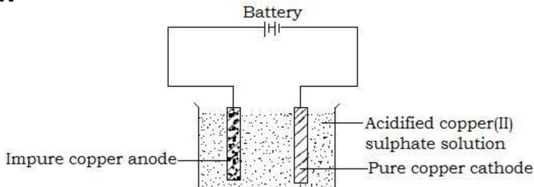
In this case, the impure metal is made the anode and the pure metal the cathode. The electrolyte is usually an acidified solution of a salt containing the metal to be purified. In this case acidified copper (II) sulphate solution is used. During electrolysis, the impure copper anode dissolves and their fore losses mass as copper (II) ions ( )are formed.
