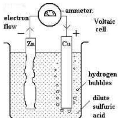
When zinc and copper strips or plate are dipped in dilute sulphuric acid then connected to an ammeter and bulb by a wire, the ammeter indicates that current is flowing.
